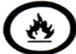
Flammable and combustible material
