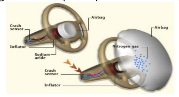
130 g of sodium azide can produce 67 litres of nitrogen gas!!!
